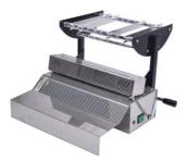
Connect AC 230 V/50 HZ power. Switch on the power switch: MS-14 will take 2 minutes to preheat Begin usage when the indicator light goes off. There are two pressure rack installment holes on each side of the machine, and you can install the pressure rack on the left or right side.
